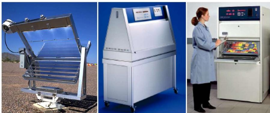
Figure 77. Equipment used to accelerate ageing phenomena: left EMMAQUE device, middle: weatherometer (sometimes called QUV chamber), Right: Xenon tester
