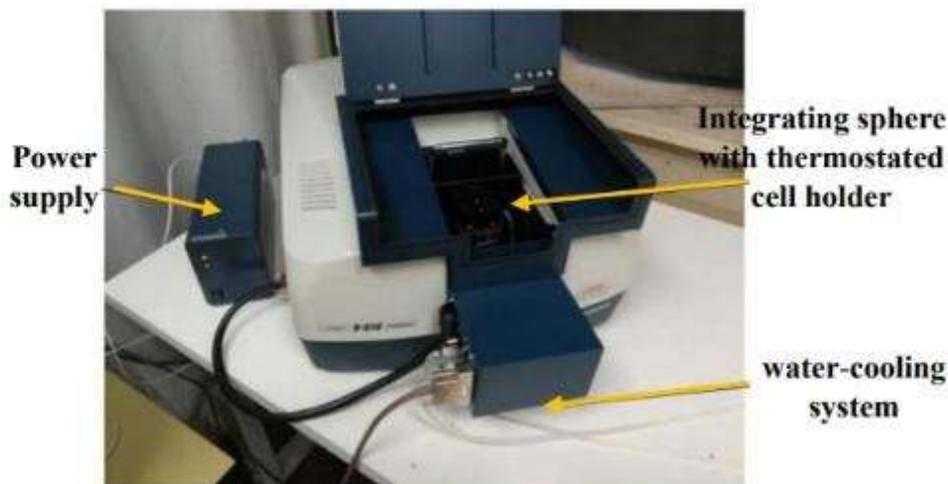
Figure 17. UV/VIS/NIR, double beam spectrophotometer Jasco V670 – Measurements of transmittance
